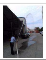
Water pressure test on Fire hydrant
